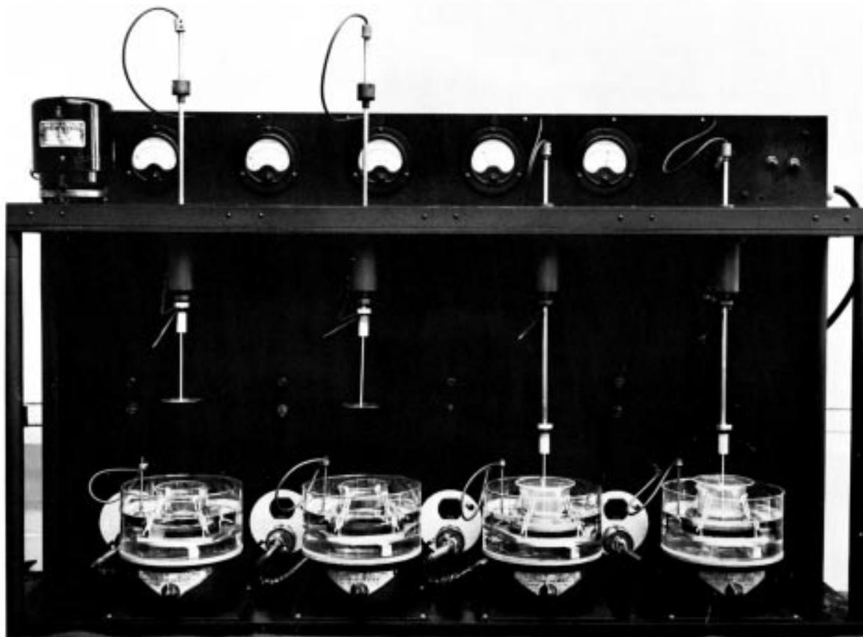
FIG. 10 Multiple-Cell Electroplating Apparatus
