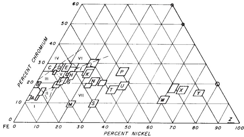
NOTE 1—The approximate areas of microstructures to be expected at room temperature are indicated as follows:
