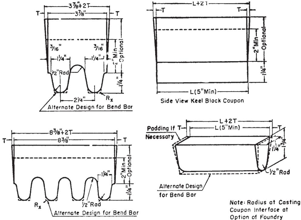
Note: Radius at Casting Coupon Interface at Option of Foundry
