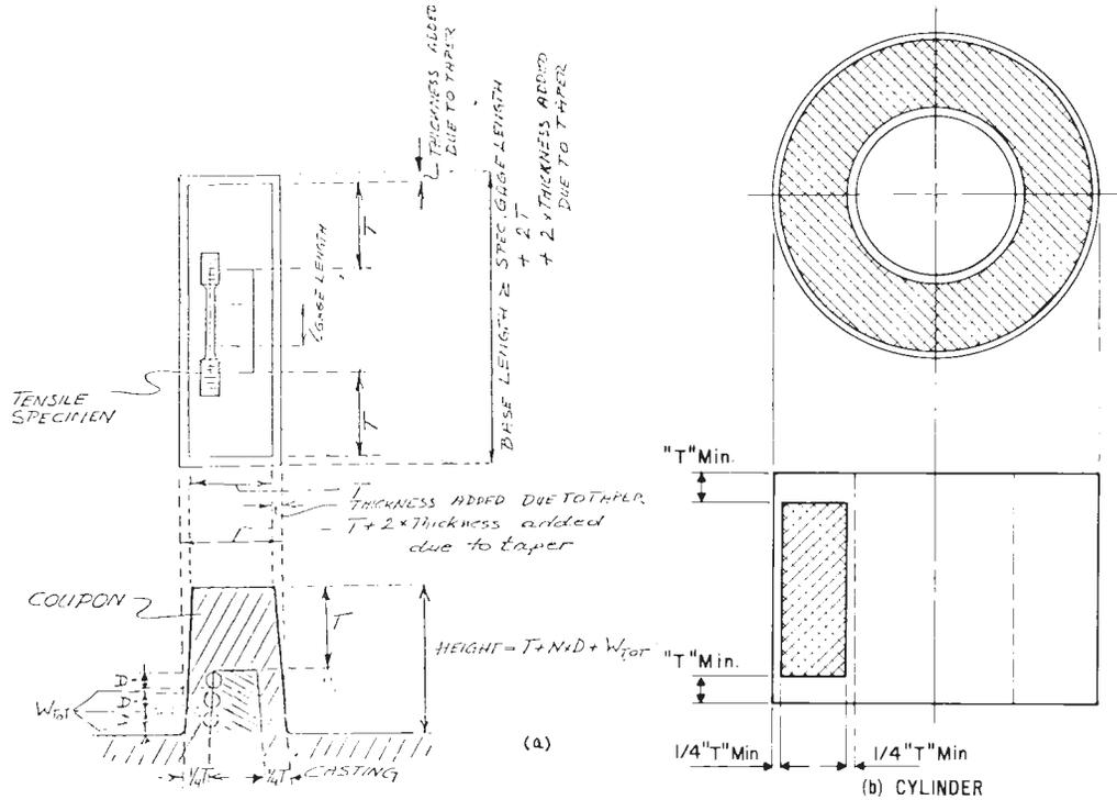
Minimum length of the base—Specimen gage length +  $2xT$  +  $2x$  the thickness due to the tapers. \
