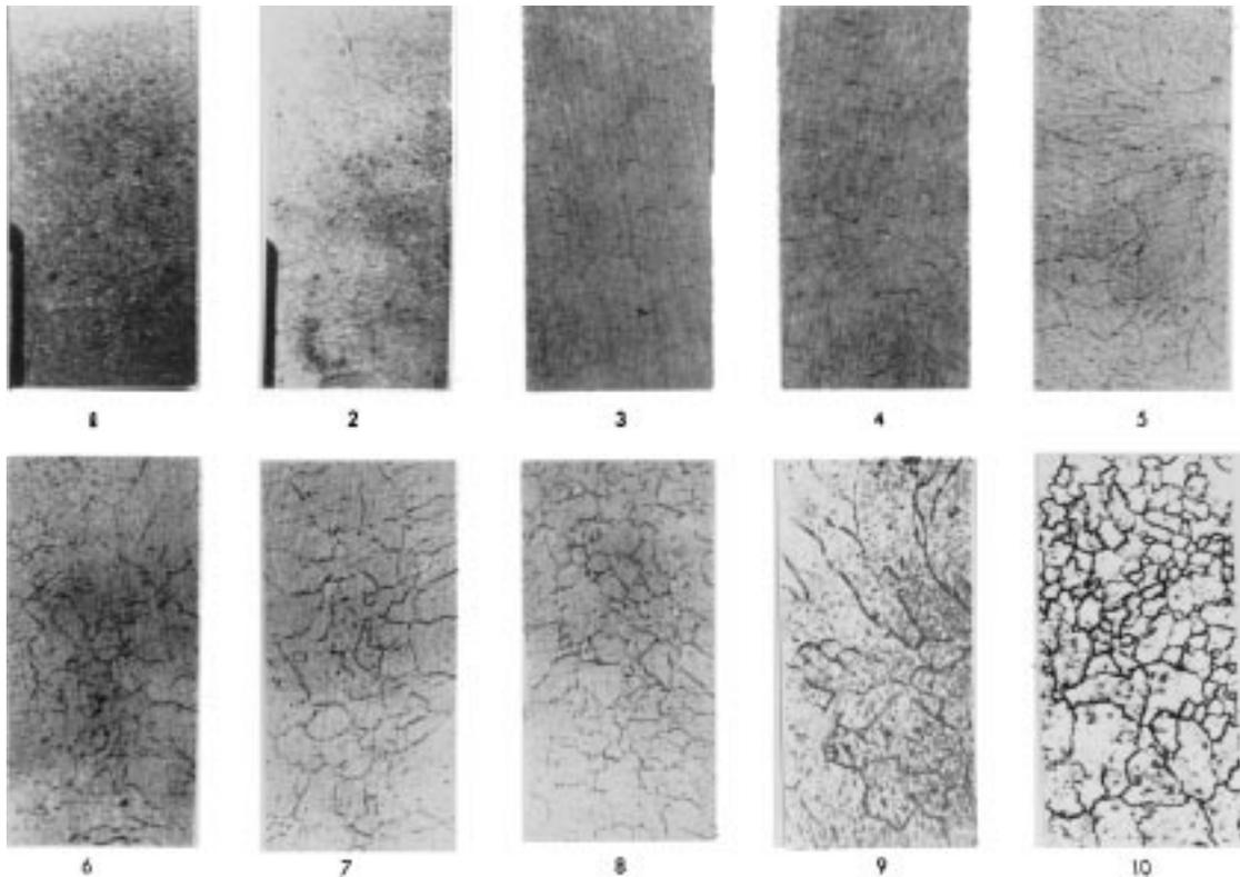
NOTE—The ten levels of severity of intergranular network structures shown are indicative of the presence of aluminum nitride precipitation in the primary austenitic grain boundaries.
