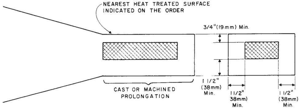
NOTE—Longitudinal axis and gage length of test specimen must be within cross-hatched zone.
