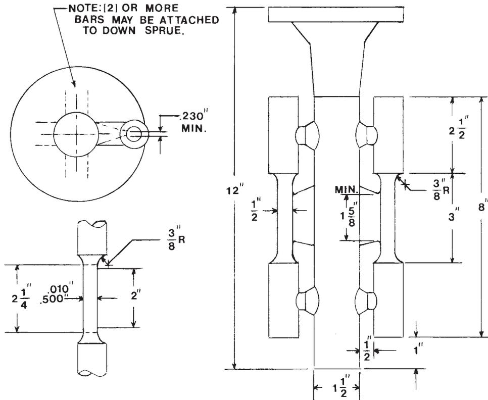
NOTE—Coupons produced in this manner are suitable for austenitic alloys only. The mold may be preheated for pouring to produce a sound coupon.
