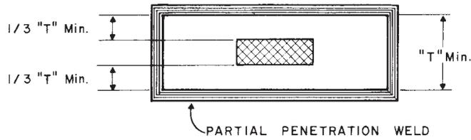
NOTE—Longitudinal axis and gage length of test specimen must be within cross-hatched zone.
