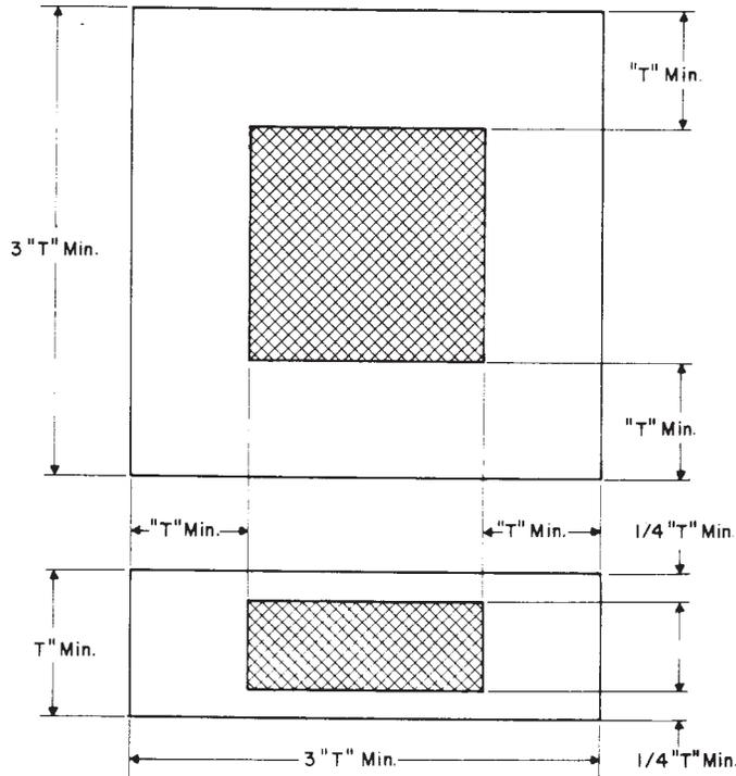
NOTE—Longitudinal axis and gage length of test specimen must be within cross-hatched zone.
