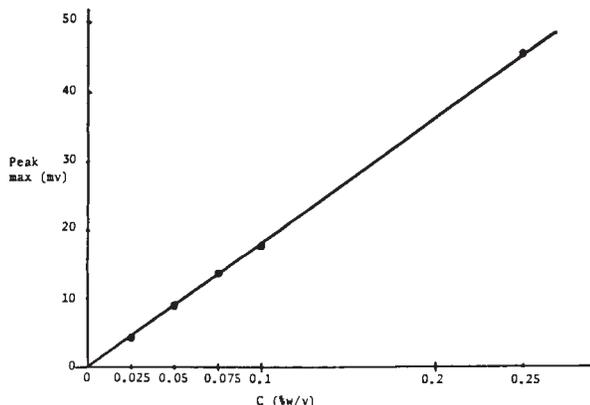
FIG. 4 Linear Detector Response to Polystyrene Sample Concentration
