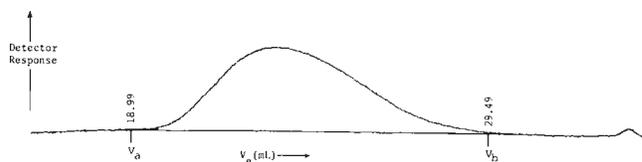
FIG. 6 Typical Chromatogram for Which This Test Method is Applicable
