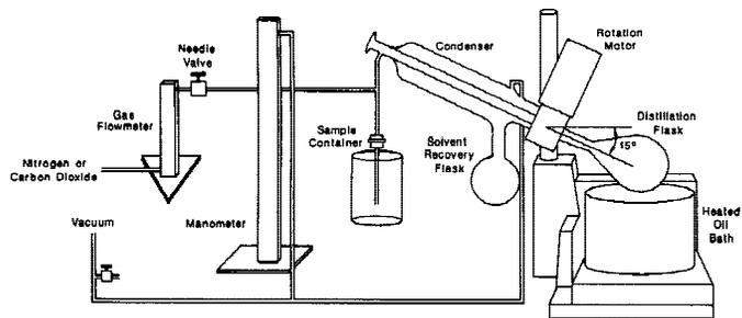
NOTE—It is important that the needle valve is at location shown; not ahead of the flowmeter.
