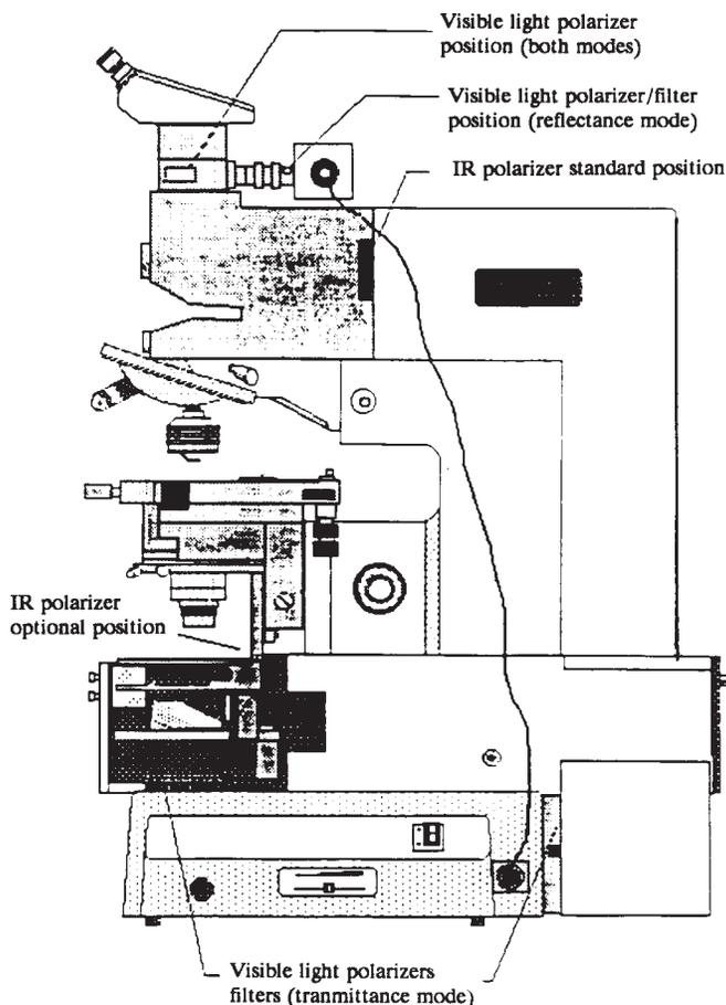
FIG. 3 Schematic Diagram of Infrared Microsampling Accessory
