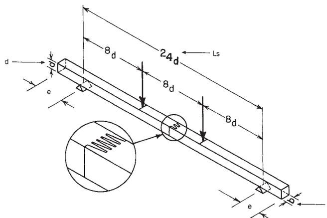
Example Dimensions for Fig. 4 Flexure Test Specimen:
