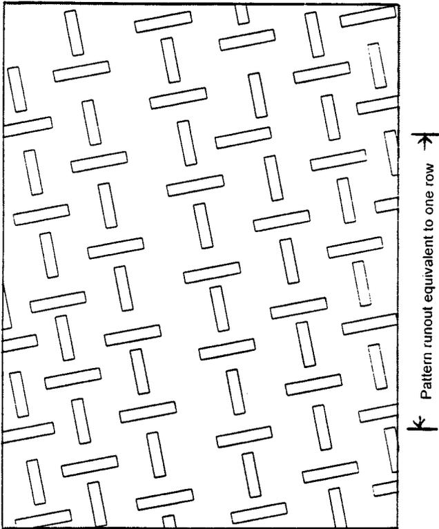
FIG. 4 Description of Pattern Runout
