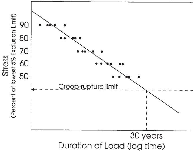
NOTE 1—Also shown is the stress or creep-rupture limit that does not cause failure with 30 years used to calculate the creep factor.
