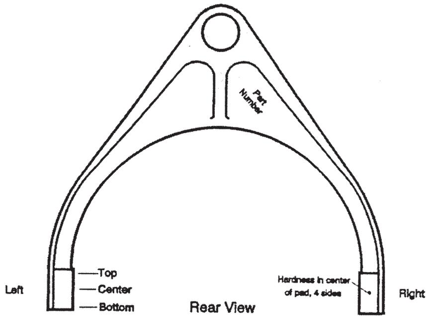
NOTE 1—Side of fork with forged angle and part number is the rear side. View the fork from this side to identify the pads as left and right.
