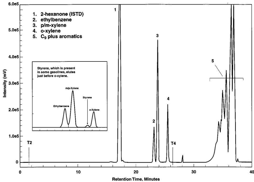
FIG. 5 Aromatics in Gasoline, Analysis No. 2
