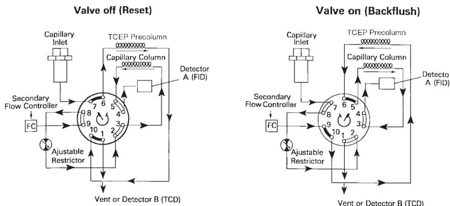
FIG. 1 Valve Diagram, Aromatics in Gasoline
