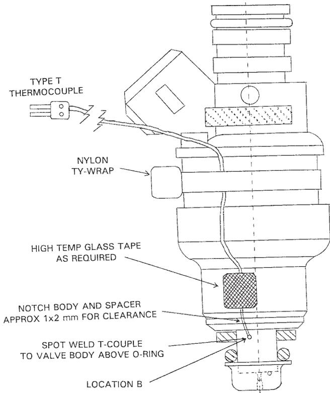
FIG. 4 Fuel Injector Skin Temperature Measurement Location
