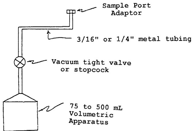
FIG. 1 Volumetric Apparatus
