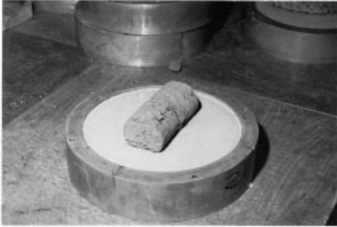
FIG. 6 Lower Half of a Specimen Encapsulated in Holding Ring
