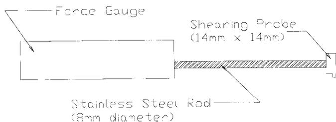
FIG. 1 Probe Design for the Detachment of Barnacles
