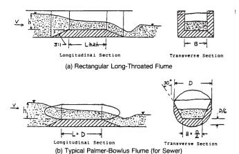
Limitations on geometry:<sup>a</sup>  $h \ge 0.15$  ft. (0.05 m)  $0.1 \le h/L \le 0.5$   $B \ge 0.33$  ft. (0.1 m) h < 6 ft. (2 m)
