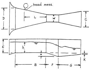
Geometry: Parshall flumes are designated by throat width, W; Standard sizes and capacities are listed as follows: Discharge equations:  ${}^{A}Q = Ch^{n}$
