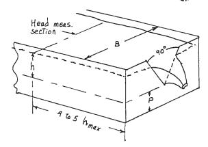
Limitations on geometry:  $^{B}$   $h/P \le 1.2$   $h/B \le 0.4$   $P \ge 0.3$  ft (0.1 m)  $P \ge 0.3$  ft (0.6 m) 0.15 ft (0.05 m)  $P \ge 2$  ft (0.6 m)
