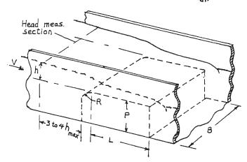
Limitations on geometry:  $\begin{array}{ll} h \geq 0.2 \; \text{ft. (0.06 \; m)} \\ R \geq 0.2 \; h_{\text{max}} \\ L \geq 1.75 \; h_{\text{max}}; \; L + R \geq 2.25 \; h_{\text{max}} \\ 0.05 \leq H/L \leq 0.57 \; (H = h + V^2/2g) \\ P \geq 0.5 \; \text{ft (0.15 \; m)} \\ H/P < 1.5 \\ B \geq 1 \; \text{ft (0.3 \; m)}; \geq H_{\text{max}}; \geq L/5 \\ \end{array}$
