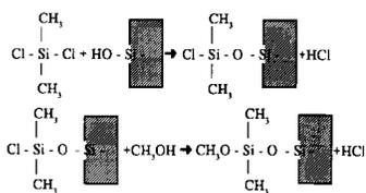
FIG. 3 Capping Silanol Groups with Dimethyl Dichlorosilane (DMDCS)
