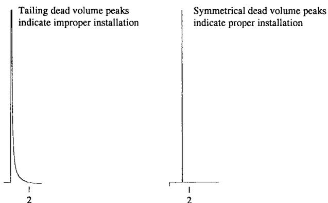
NOTE 1—Non-retained compounds such as methane that show tailing indicate a system or installation problem that must be corrected before using the column analytically.
