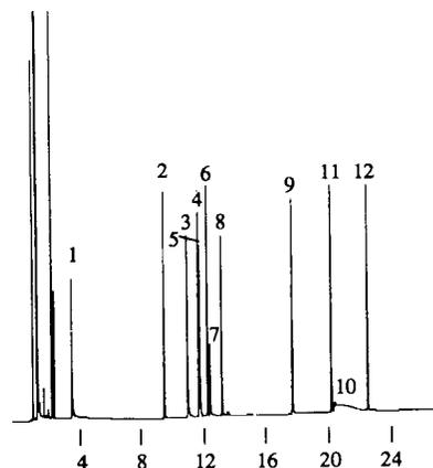
NOTE 1—The Grob mix on this column shows poor performance. Tailing 2,3-butanediol, octanol, and dicyclohexylamine peaks may indicate inadequate split/splitless sleeve deactivation. Asymmetrical hydrocarbon and FAME peaks may indicate that the column has been installed improperly.
