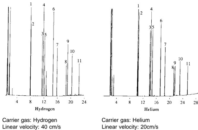
NOTE 1—Hydrogen is only slightly faster than helium when both carrier gases are operated under the same temperature-programmed oven conditions.
