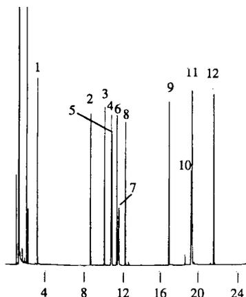
NOTE 1—The Grob mix shows that this column is performing adequately. Symmetrical hydrocarbon and FAME peaks indicate that the column has been installed properly (that is, no dead volume exists in column connection). Active probes such as 2,3-butanediol, octanol, nonanal, and dicyclohexylamine are symmetrical which indicates adequate deactivation of split/splitless sleeves.
