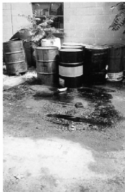
**FIG. X2.12 Surface Staining from Improper Drum Storage**
