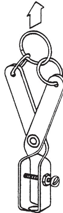
FIG. 9 Tension Test Adapter/Clamp
