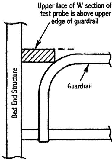
FIG. 7 (a) Partially Bounded Opening (Conforms to Requirement)
