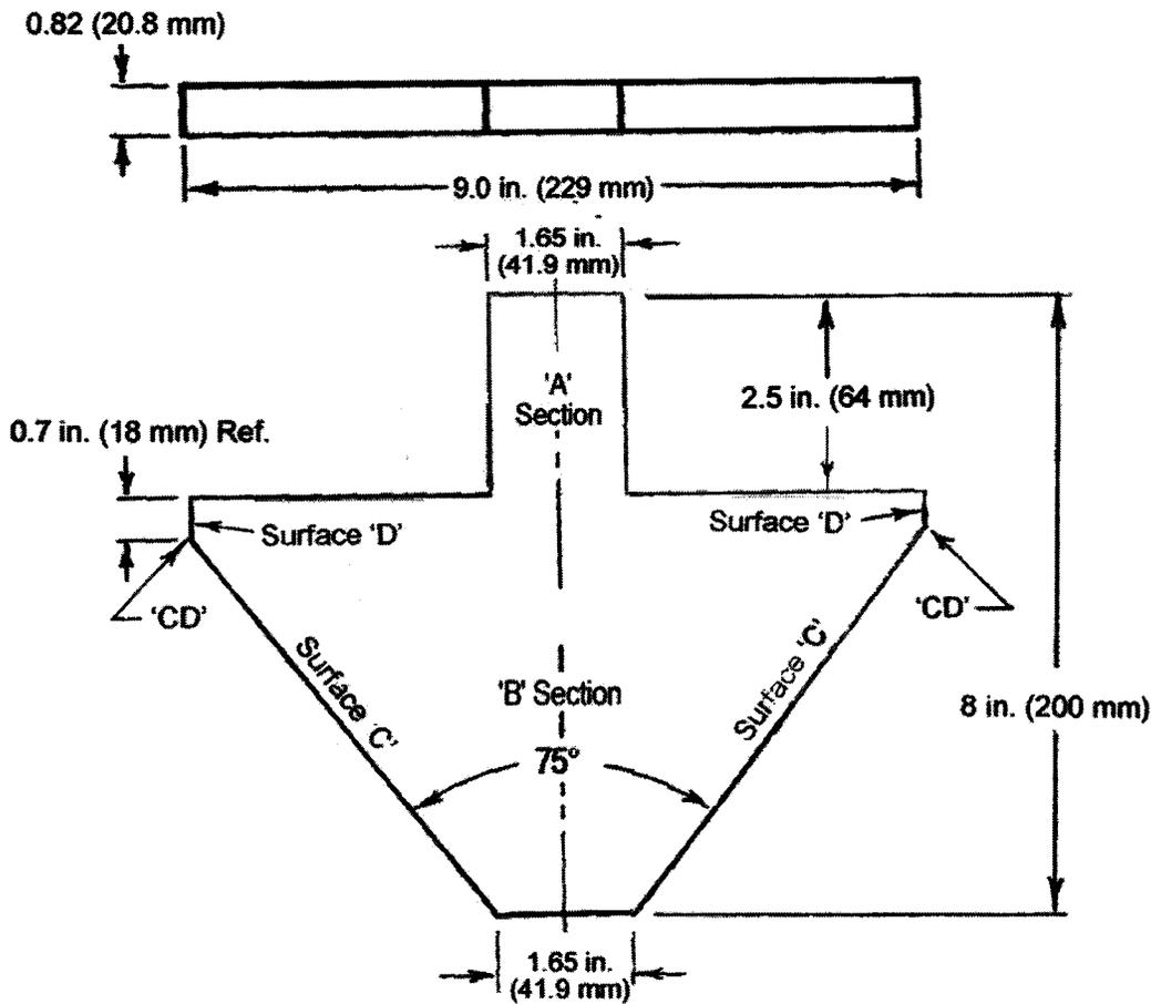
**Probe to be made of any rigid material**
