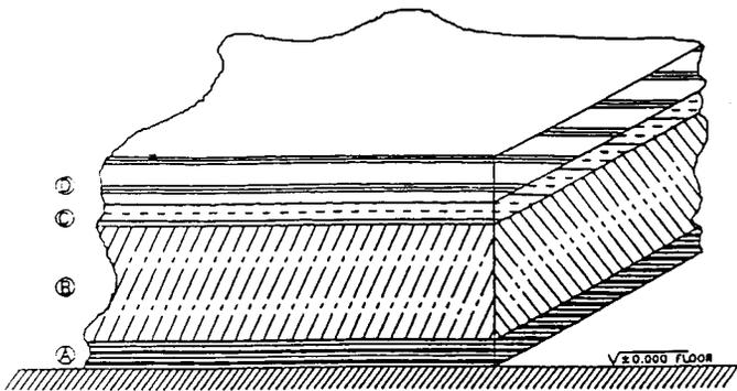
NOTE 1—(A) Poly(methyl methacrylate) sheet,  $0.25 \pm 0.03$ -in. ( $6 \pm 0.1$ -mm) thickness; (B) AC exterior glue fir plywood sheet,  $0.75 \pm 0.08$  in. ( $19 \pm 0.2$  mm) or greater in thickness; (C) polypropylene microfoam sheet;  $0.7 \pm 0.01$ -lb/ft<sup>3</sup> ( $11 \pm 0.2$ -kg/m<sup>3</sup>) density and  $0.13 \pm 0.01$ -in. ( $3 \pm 0.03$ -mm) thickness; and (D) glass/tempered sheet,  $0.38 \pm 0.04$ -in. ( $10 \pm 0.1$ -mm) thickness.
