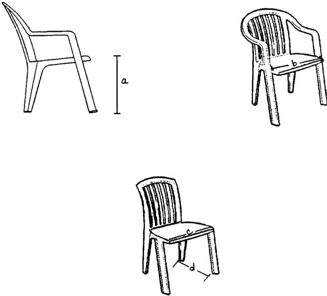
NOTE 1—(a) Seat height, chair with or without arms; (b) seat width, chair with arms; and (c) seat width, chair without arms; (d) leg stance, measured from back of front leg to back of rear leg.
