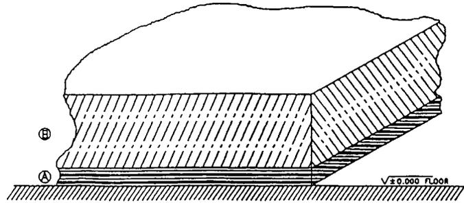
NOTE 1—(A) Poly(methyl methacrylate) sheet,  $0.25 \pm 0.03$ -in. ( $6 \pm 0.1$ -mm) thickness; and (B) AC exterior glue fir plywood sheet,  $0.75 \pm 0.08$  in. ( $19 \pm 0.2$  mm) or greater in thickness.
