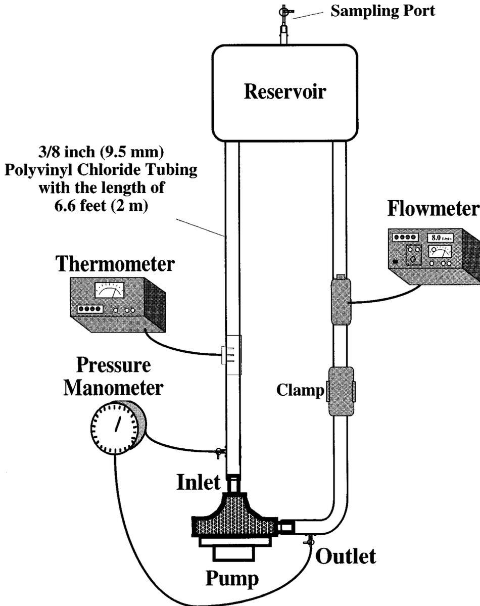
FIG. 1 Test Loop
