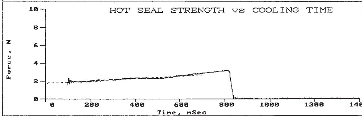
FIG. 2 Cooling Curve
