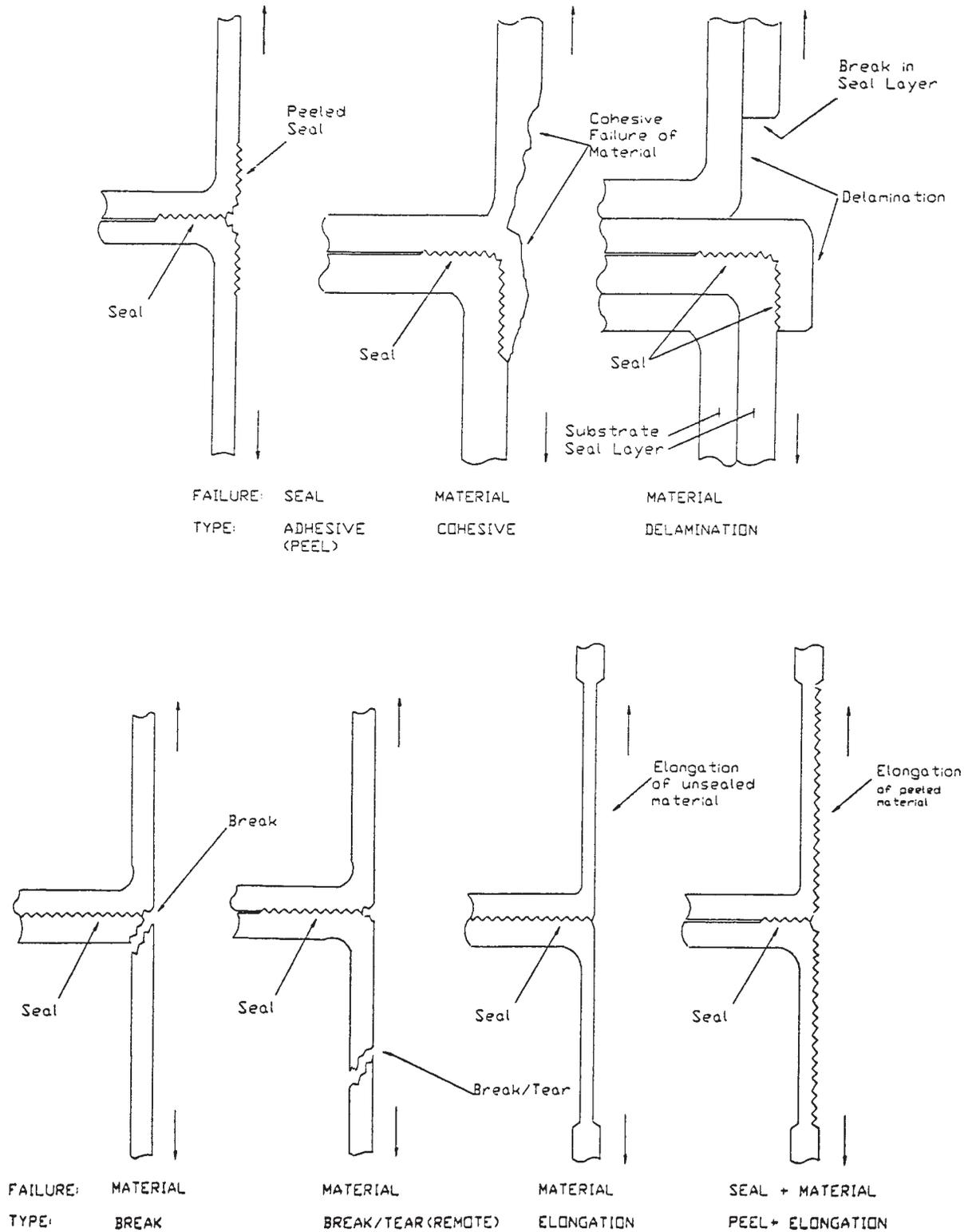
FIG. 1 Test Strip Failure Modes
