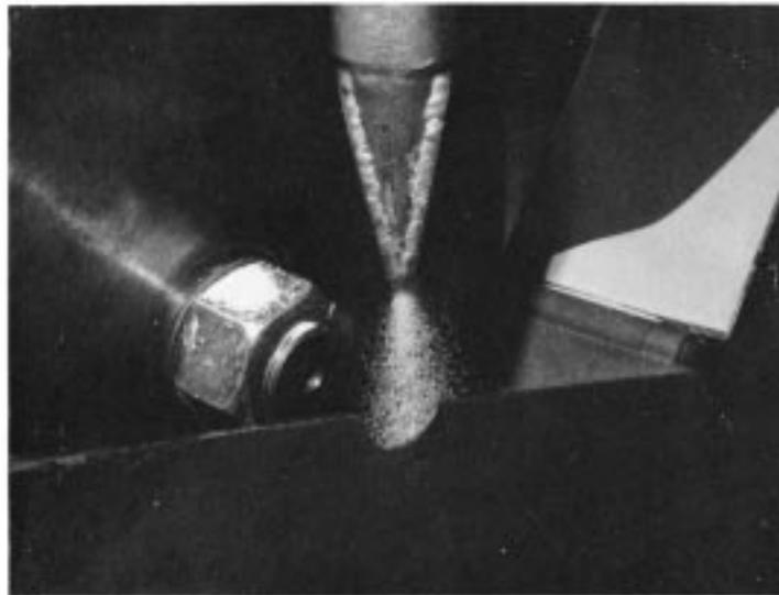
FIG. 10 Sand Flow—Turbulence
