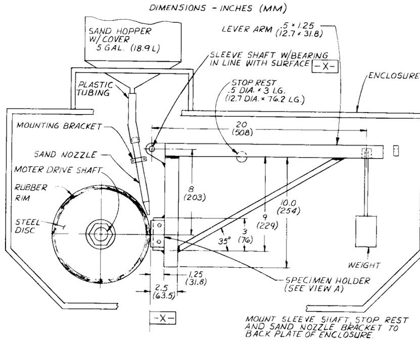
FIG. 2 Dry Sand/Rubber Wheel Abrasion Test Apparatus
