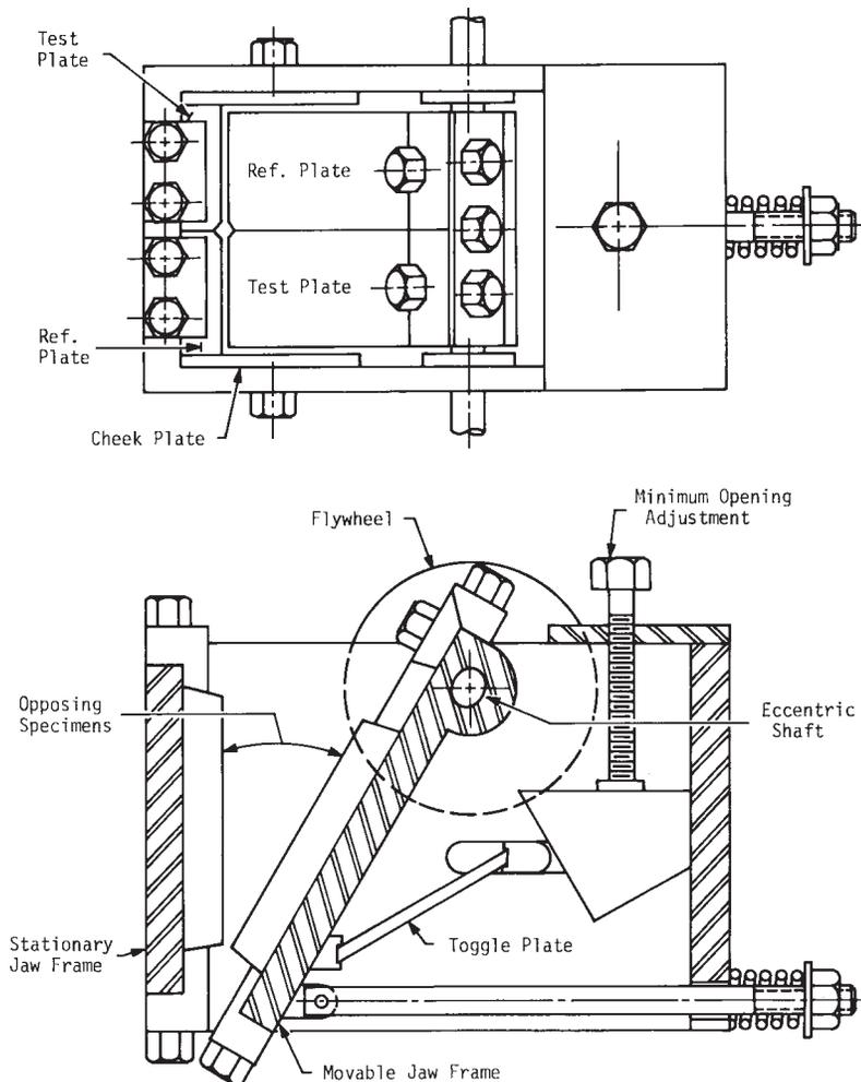
FIG. 1 Typical Jaw Crusher Construction and Layout of the Test Plates
