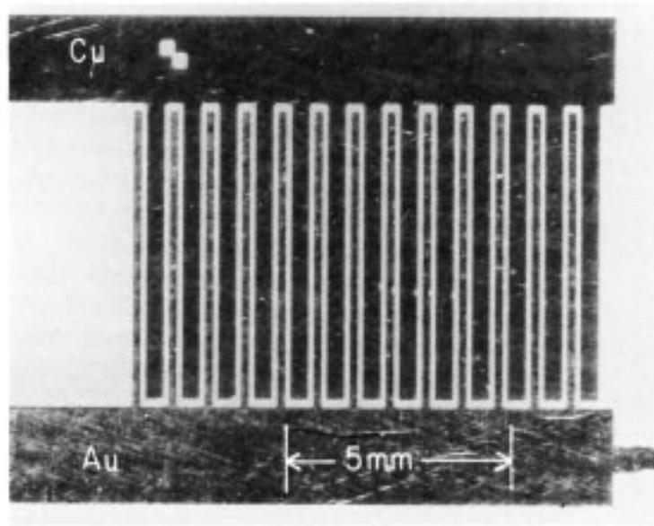
FIG. 1 Sensing Element
