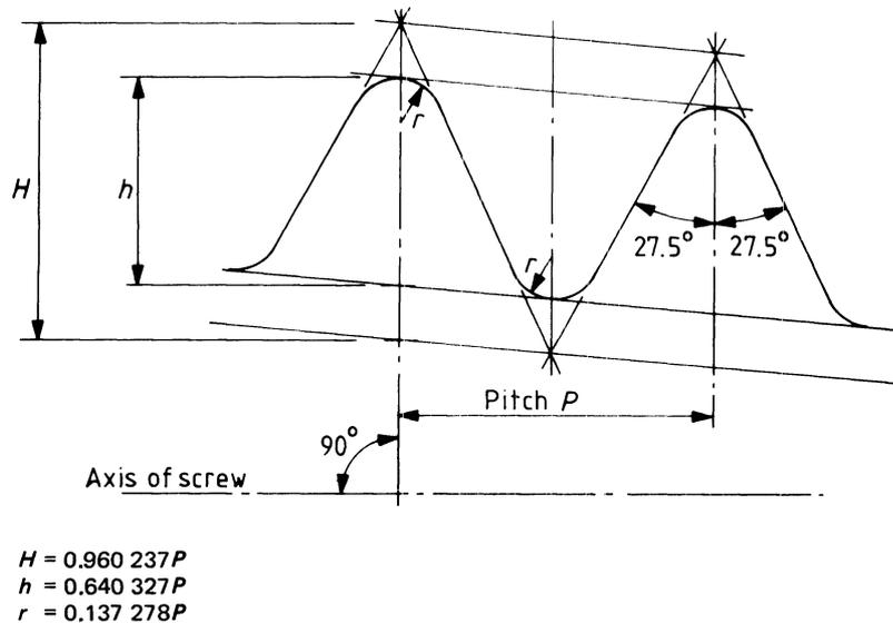
NOTE The taper is 1 in 16 measured on the diameter (shown exaggerated in the diagram).
