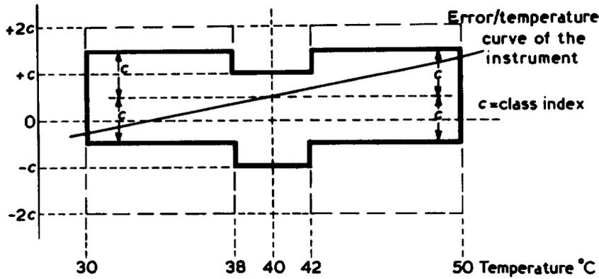
Figure 4 — Effect of temperature. Reference value  $40\text{ }^{\circ}\text{C}$
