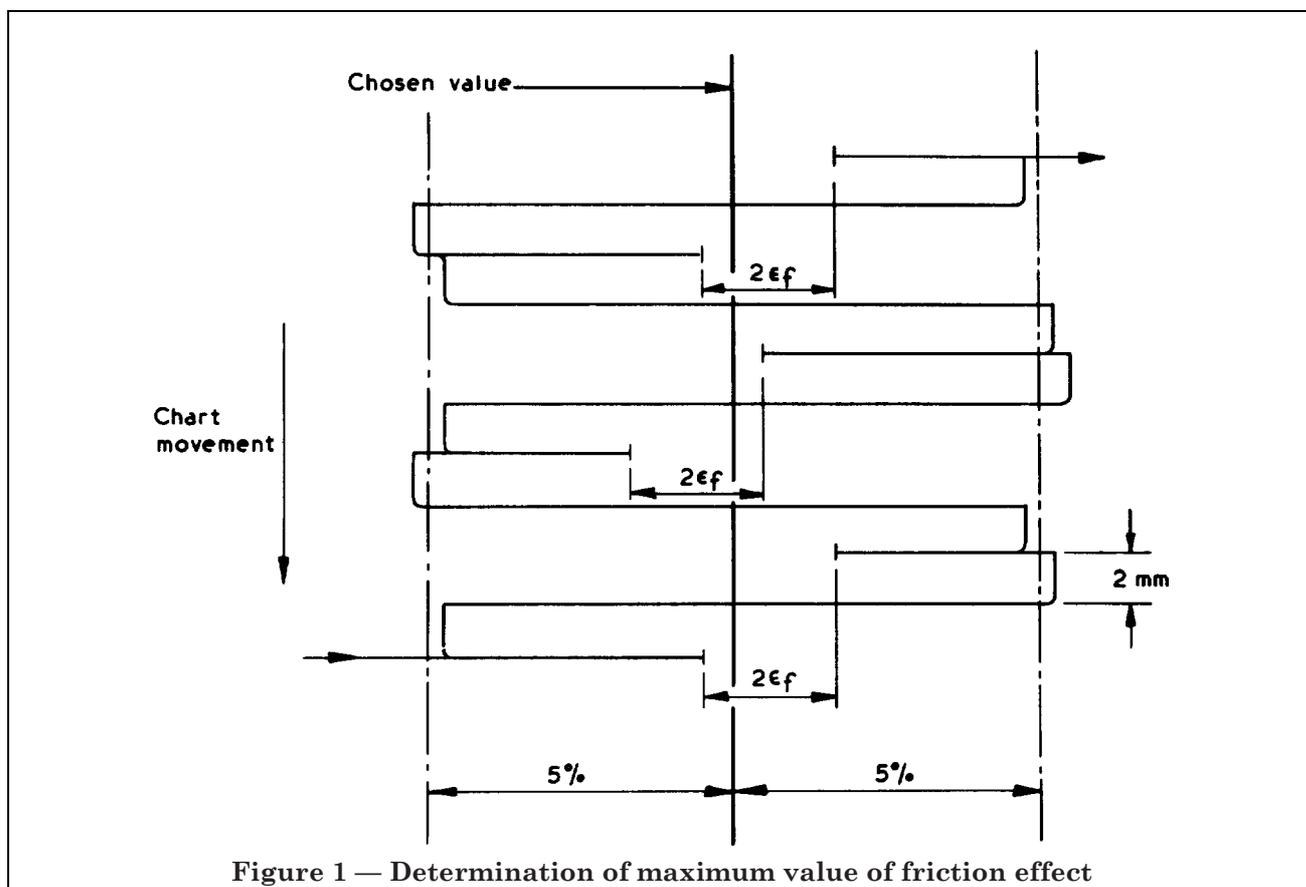
**9.2.2** The maximum value of friction effect determined according to 9.2.1 shall not exceed the limit which is specified by the manufacturer and marked on the instrument (symbol K-1 of Table 17).
