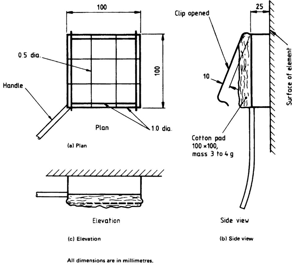
Figure 5 — Typical frame for supporting for cotton pad
