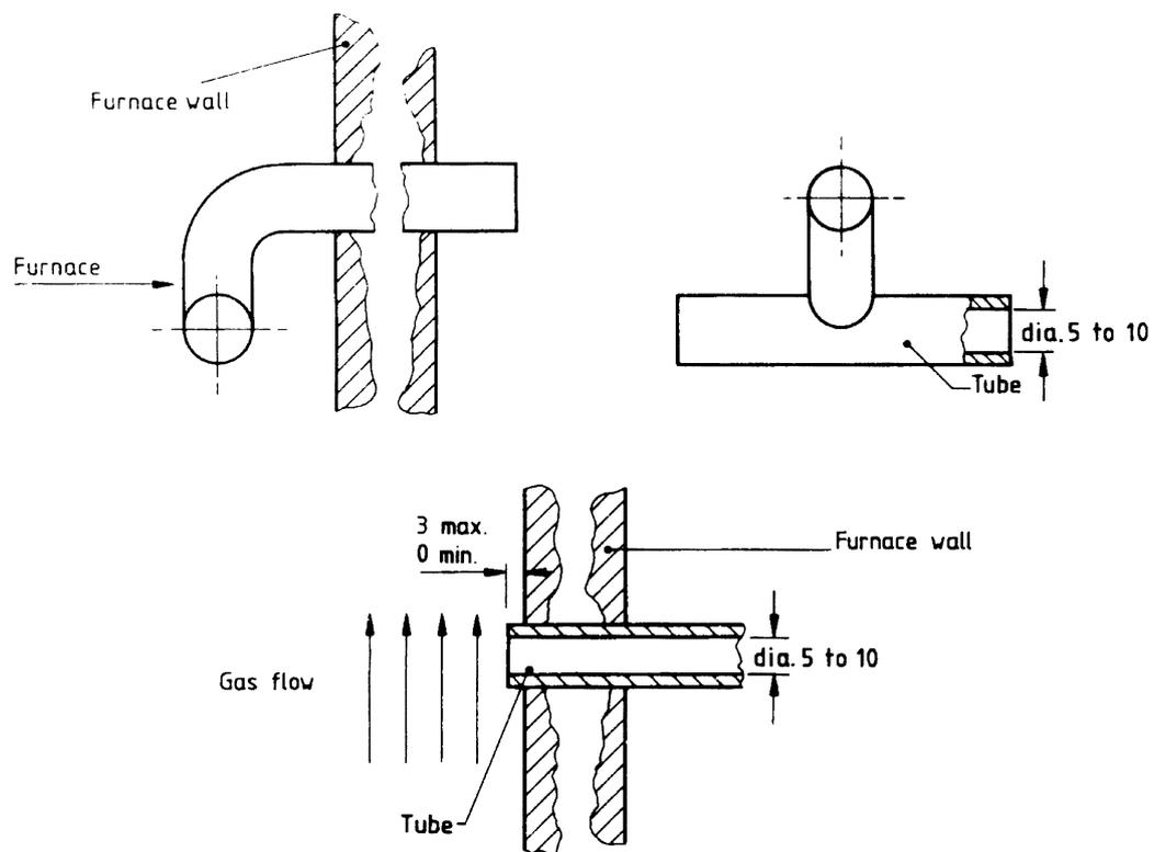
Figure 8 — Pressure sensing head
