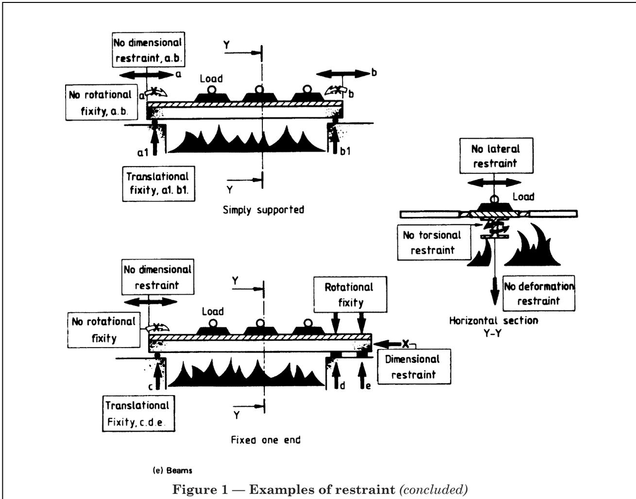
Figure 1 — Examples of restraint (concluded)
