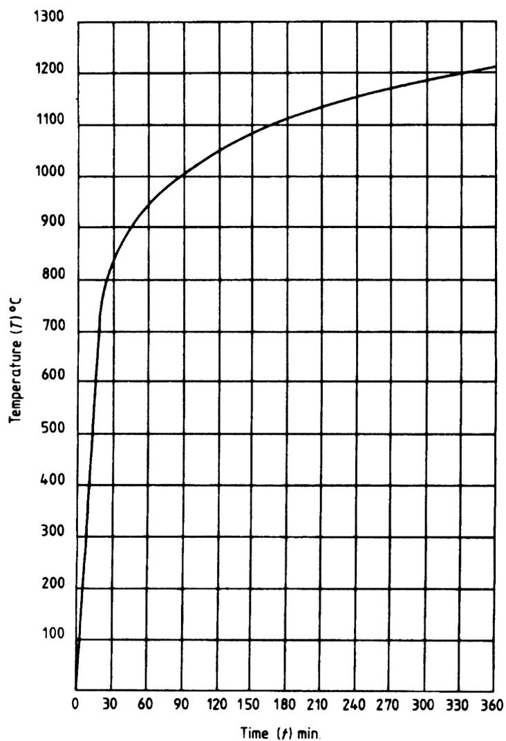
Figure 2 — Standard temperature/time curve
