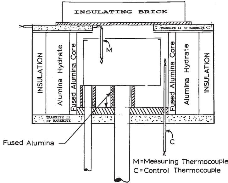
NOTE 1—Heating elements attached to fused alumina core—covered with baked-on refractory cement.
