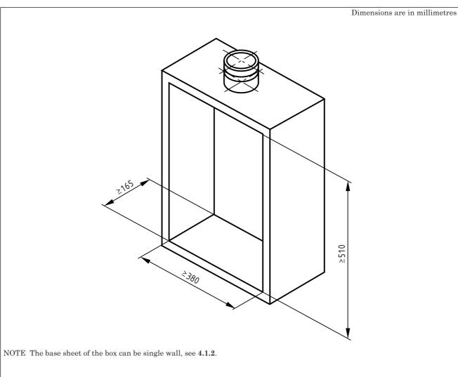
$Figure \ 1 - Dimensions \ of \ a \ flue \ box \ for \ a \ typical \ gas-fired \ radiant/convector \ and \ live \ fuel \\ effect \ fire$
