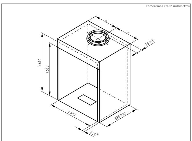
NOTE Except for those given in this figure, dimensions are to suit the appliance manufacturer. Gap between inner and outer walls to be 25 mm minimum.
