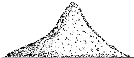
b) Aggregate slightly moist; appreciable slump observed
