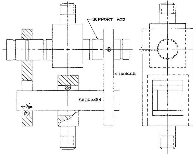
**FIG. 1 Suggested Bearing Edge and Specimen Support**
