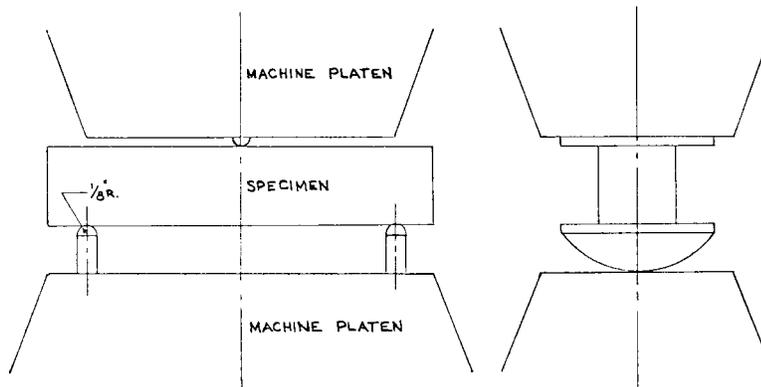
**FIG. 2 Alternative Suggested Bearing Edge and Specimen Support**
