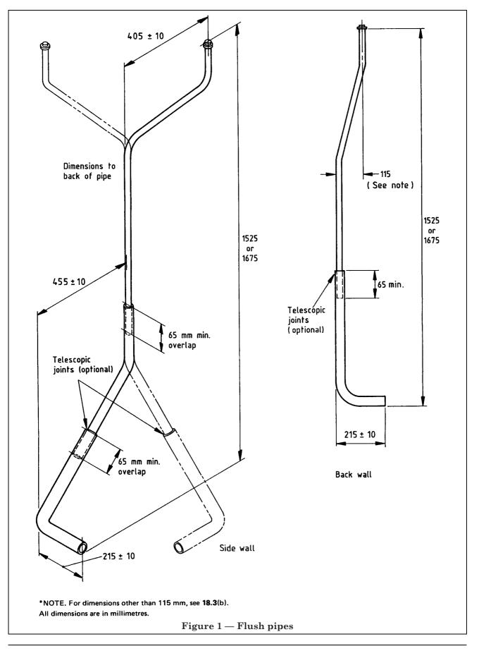
**18.3** The centre of the outlet shall be central in the width and, except for cisterns intended solely for low-level use, shall be either:
