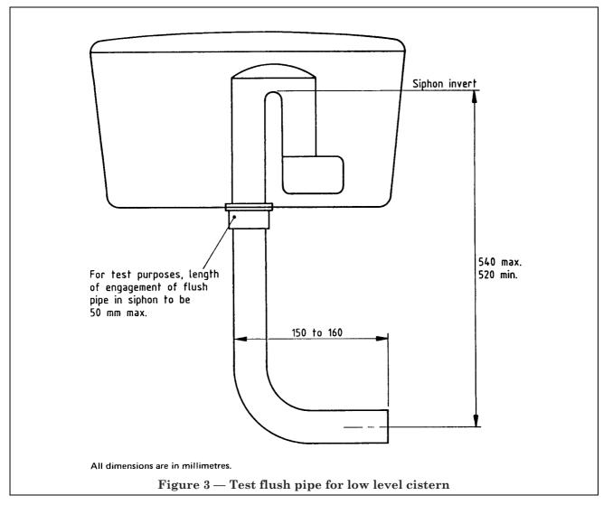
**E.2.3** Procedure for low level cisterns. At the end of 6.5 s, or a computed shorter period if the volume of discharge is less than 9 L, rapidly draw the vessel clear or otherwise divert the flow of water and ascertain, either by measuring or weighing, the volume of water collected in the vessel (see clause 10).
