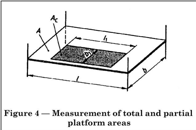
Figure 4 — Measurement of total and partial platform areas
