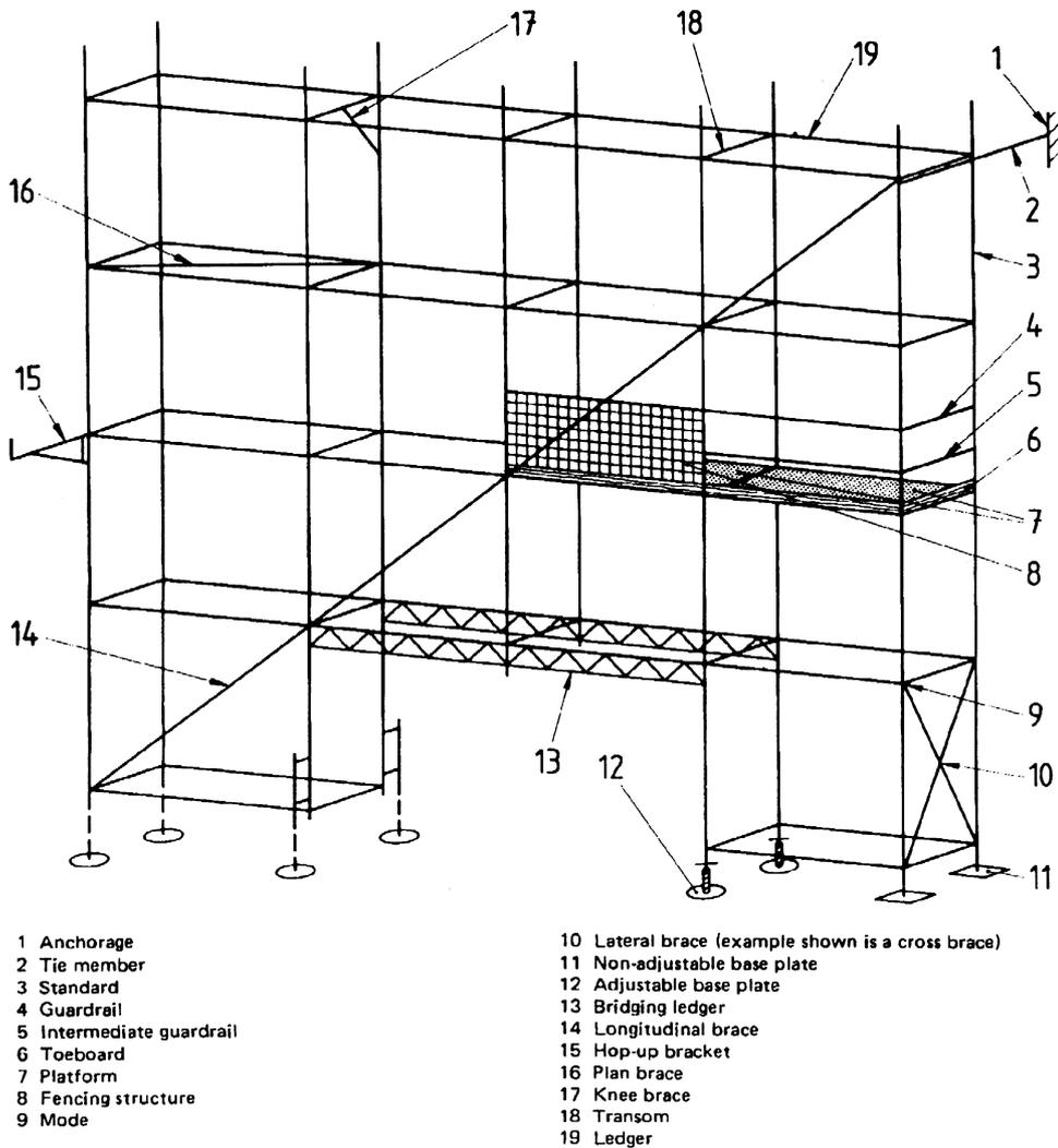
**Figure 1 — Identification of typical components of a prefabricated scaffold system**
