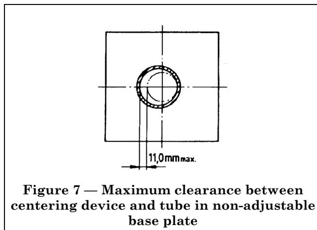
Figure 7 — Maximum clearance between centering device and tube in non-adjustable base plate
