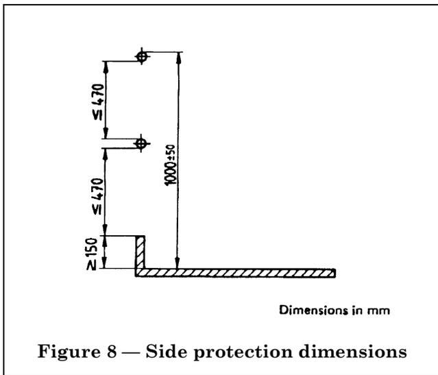
Figure 8 — Side protection dimensions
