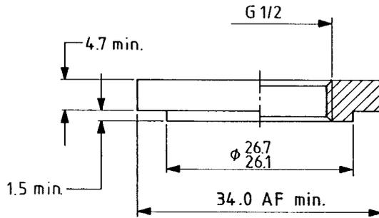
(b) Type (b) size  $\frac{1}{2}$  backnut (spigoted)
