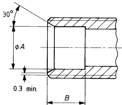
(c) Inlet (bottom or side entry) for connection to 12 mm or 15 mm copper tube (see clause 13.4)
