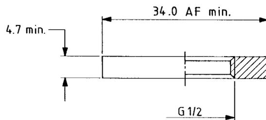
(c) Type (c) size  $\frac{3}{8}$  and  $\frac{1}{2}$  backnuts (fixed flange)
