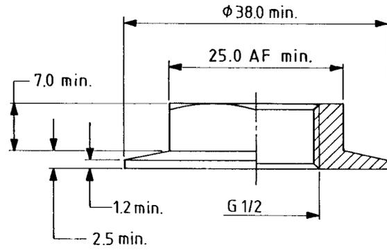
(a) Type (a) size  $\frac{3}{8}$  and  $\frac{1}{2}$  backnuts (integral flange)
