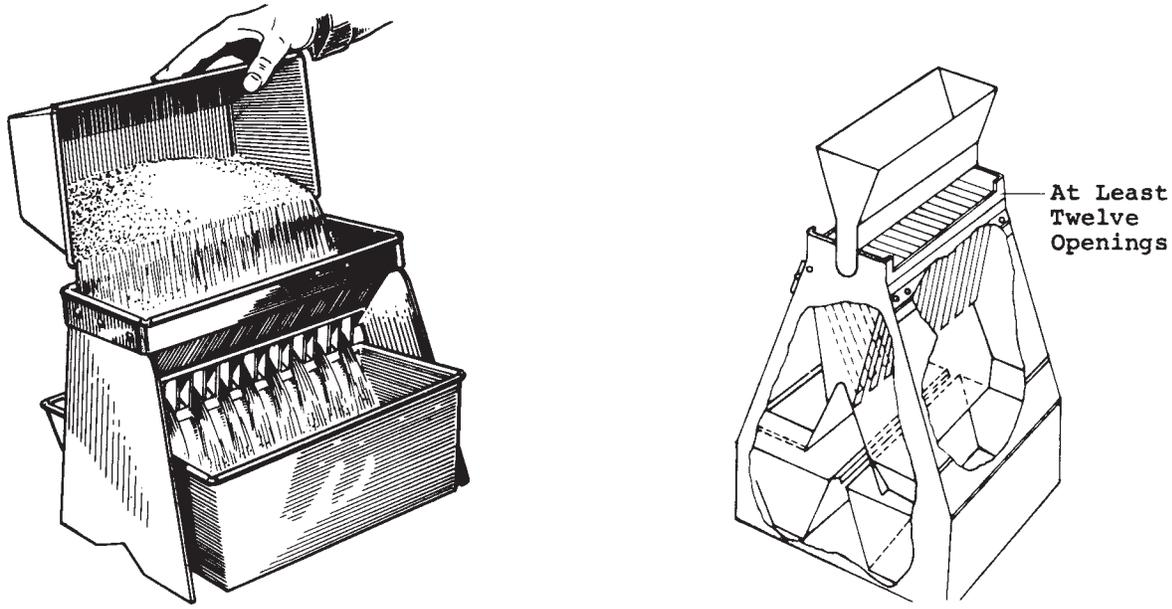
NOTE— Small Sample Splitters for Fine Aggregate. May be constructed as either closed or open type. Closed type is preferred.
