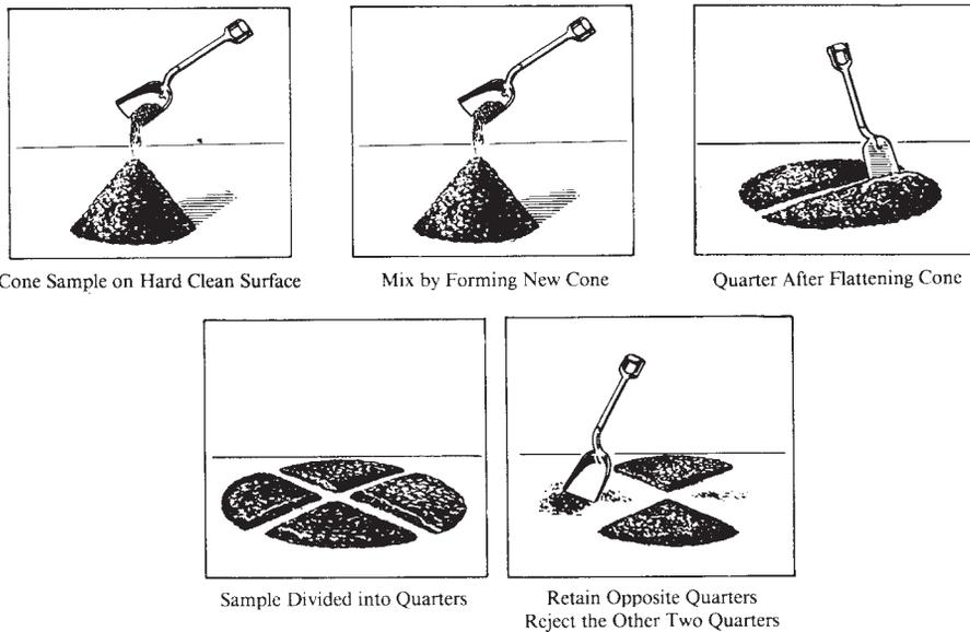
FIG. 3 Quartering on a Hard, Clean Level Surface
