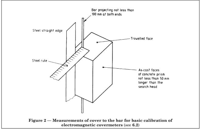
The concrete should have an ordinary Portland cement content between 300 kg/m³ and 400 kg/m³ and the aggregate should not have significant magnetic properties. No additions should be used in the concrete. Care should be taken during casting not to bend the bar.
