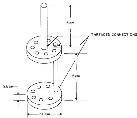
FIG. 2 TFE-Fluorocarbon Cage for 100-mL Test Tube
