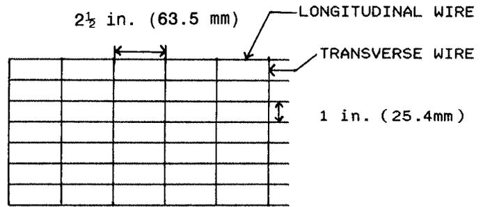
FIG. 4 Type WW-S—Welded Mesh with Straight Longitudinal Wires
