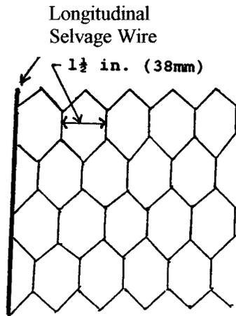
FIG. 1 Type TW—Twisted Hexagonal Mesh (Design Number 7.5 × 0 × 0.054 × 0)
