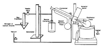
NOTE-It is important that the needle valve is at location shown; not ahead of the flowmeter.
