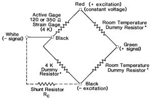
FIG. 3 A Method of Strain-Gage Wiring for Cryogenic Tests
