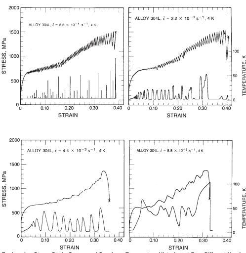
FIG. 2 Typical Engineering Stress-Strain Curves and Specimen Temperature Histories, at Four Different Nominal Strain Rates, for AISI 304L Stainless Steel Tested in Liquid Helium (4)
