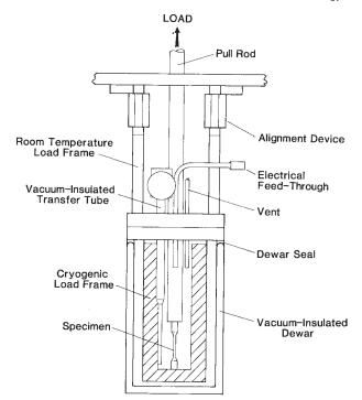
FIG. 1 Schematic Illustration of Typical Cryostat for Tension Testing at 4 K
