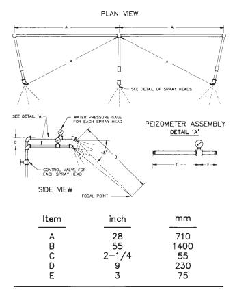
FIG. 8 Rain Test Spray-Head Piping
