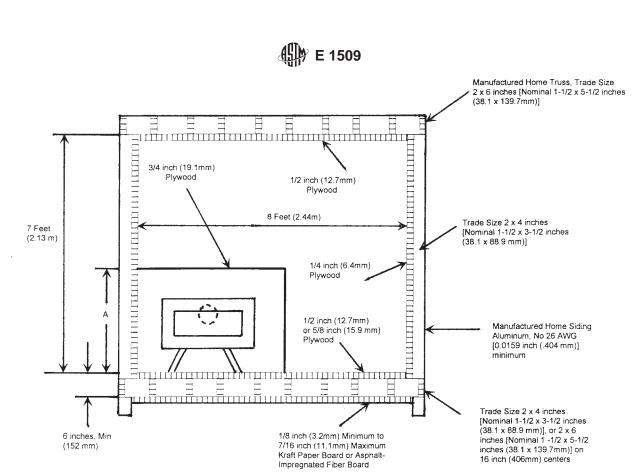
FIG. 1 Combined Conventional Home and Manufactured Home Test Structure (Shown with Optional Alcove Test Enclosure); Installation with a Direct Exhaust Venting System and Optional Alcove Enclosure
