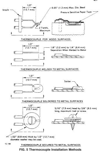
9.13 Thermocouples shall be placed on surfaces of the test structure at locations that will measure maximum temperatures during tests. A minimum number of typical thermocouple locations are shown in Fig. 6.
