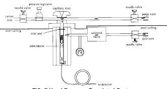
FIG. 7 Head Pressure Regulated System
