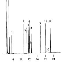
NOTE 1-The Grob mix on this column shows poor performance. Tailing 2,3-butanediol, octanol, and dicyclohexylamine peaks may indicate inadequate split/splitless sleeve deactivation. Asymmetrical hydrocarbon and FAME peaks may indicate that the column has been installed improperly.
