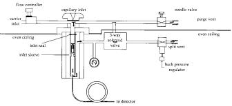
FIG. 6 Flow-Regulated Back Pressure System
