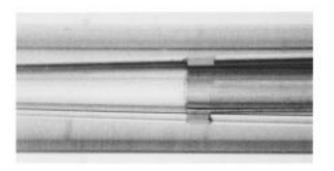
NOTE 1—A proper seal is made when a continuous ring forms at the column end and connector mating point.
