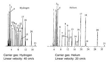
NOTE 1—Fig. 2 shows that the resolution is similar but the analysis time is reduced by 50 % when comparing hydrogen to helium in an isothermal analysis using optimum flow velocities.
