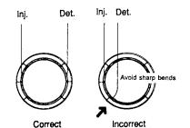
FIG. 10 Avoid Sharp Bends When Installing Fused Silica Capillary Column
