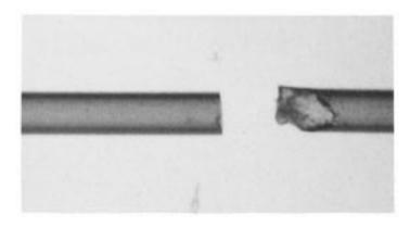
NOTE 1—This photo shows a good and bad column cut. The good cut leaves the end of the column square and free of fragments or fractures. FIG. 8 Good Versus Bad Column Cut
