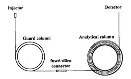
NOTE 1—A guard column protects the analytical column from damage by nonvolatile residue, particulates, or derivatization. FIG. 15 Fused Silica Guard Column
