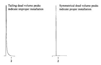
NOTE 1—Non-retained compounds such as methane that show tailing indicate a system or installation problem that must be corrected before using the column analytically.
