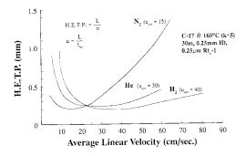
NOTE 1—The curves were generated by plotting the height equivalent to a theoretical plate (length of column divided by the total number of theoretical plates, H.E.T.P.) against the column's average linear velocity. The lowest point on the curve indicates the carrier gas velocity in which the highest column efficiency is reached.
