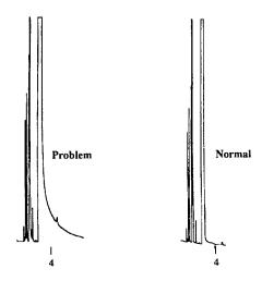
NOTE 1—The shape of the solvent peak is a good indicator of system integrity.
