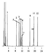
NOTE 1—The Grob mix shows that this column is performing adequately. Symmetrical hydrocarbon and FAME peaks indicate that the column has been installed properly (that is, no dead volume exists in column connection). Active probes such as 2,3-butanedial, octanol, nonanal, and dicyclohexylamine are symmetrical which indicates adequate deactivation of split/splitless sleeves.
