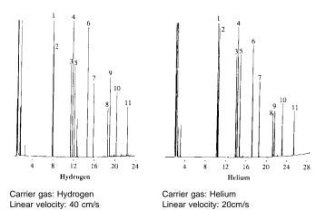
Note 1—Hydrogen is only slightly faster than helium when both carrier gases are operated under the same temperature-programmed oven conditions.
