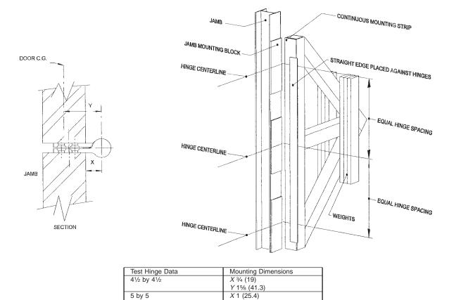
FIG. X1.1 Typical Cycle Test Apparatus
