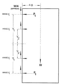
FIG. X2.2 Forces Acting on Oversized Door
