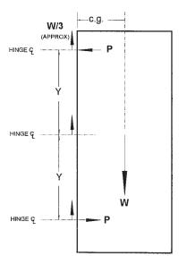
FIG. X2.1 Forces Acting on Standard-Size Door
