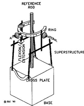
FIG. 3 Attachment of Halo Superstructure
