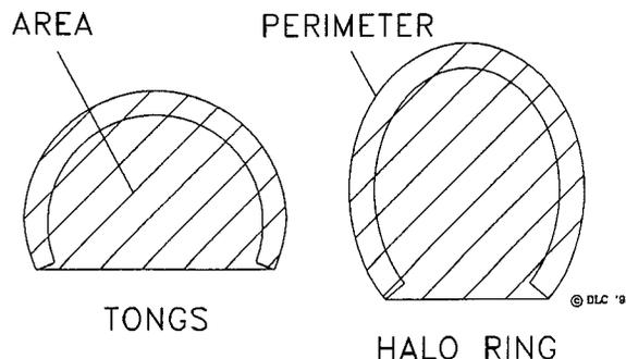
**FIG. 4 Area and Perimeter of Conductive Loop**
