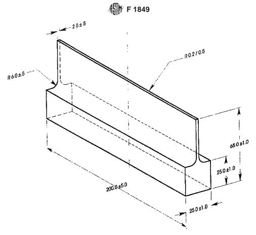
Note 1—All dimensions in millimetres. FIG. 1 Skate Blade Anvil
