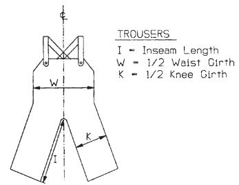
FIG. X1.2 Trouser Measurements
