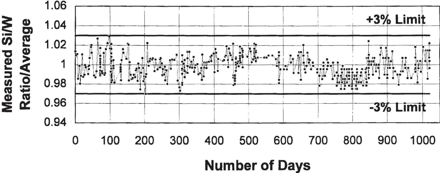
NOTE 1—Since the values were obtained from various samples with widely varying compositions, the ratios are normalized by originally measured silicon/tungsten ratios.
