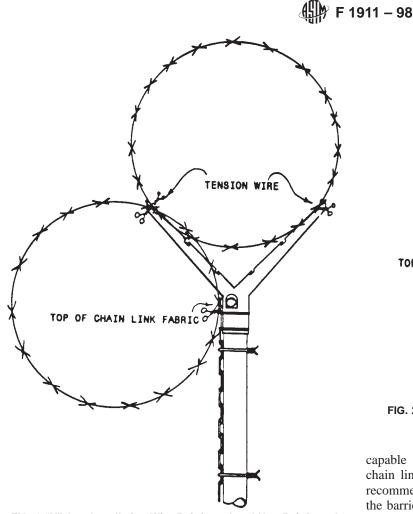
FIG. 1 "V" Arm Installation Wire-Reinforced and Non-Reinforced Barbed Tape Concertina.
