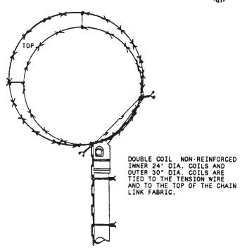
FIG. 5 Top of the Fence 45° Barb Arm Installation
