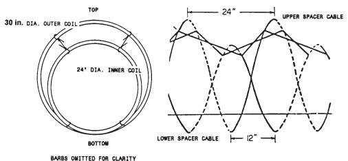
FIG. 4 Double Coil Non–Reinforced
