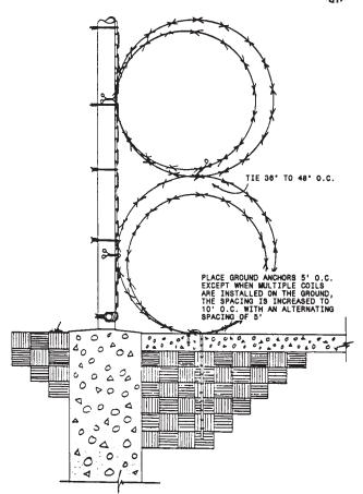
FIG. 9 Side and Bottom of Fence Installation Wire Reinforced Double Coil Concertina
