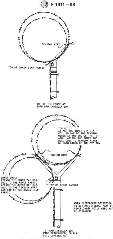
FIG. 8 Wire Reinforced Double Coil Concertina
