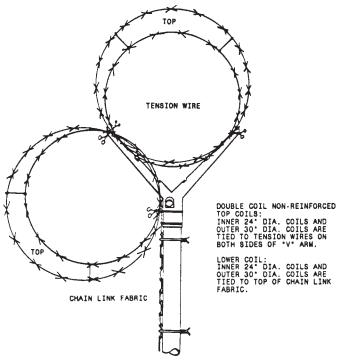
FIG. 6 Top of the Fence "V" Arm Installation
