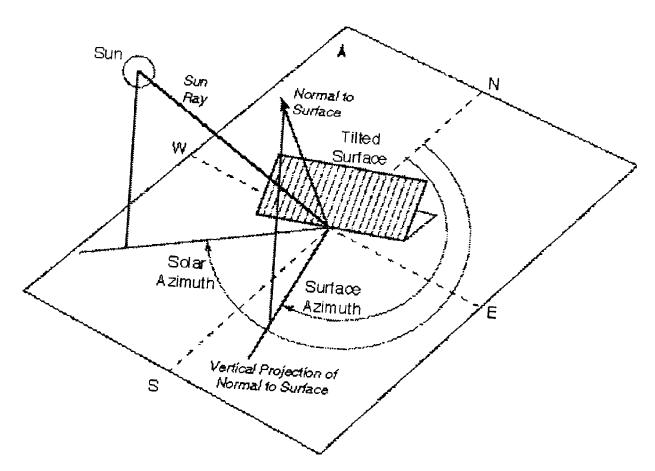
FIG. 1 Solar Azimuth Angle
