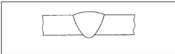
Figure 103 Root concavity
