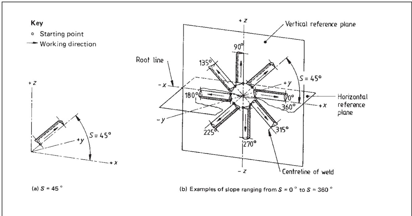
Figure 56 Schematic diagram of main welding positions
