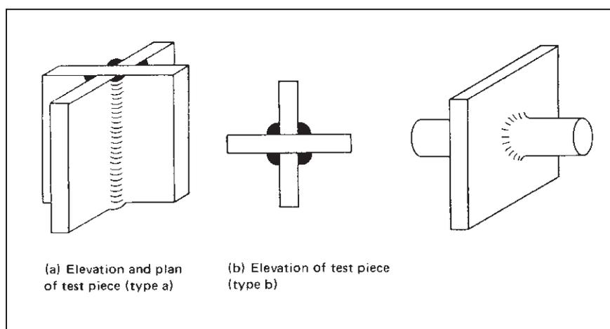
Figure 93 Method of obtaining cruciform test specimen
