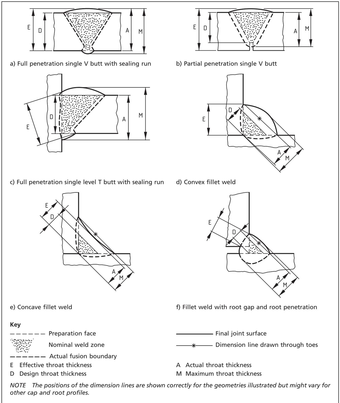
Figure 54 Examples of excess weld metal
