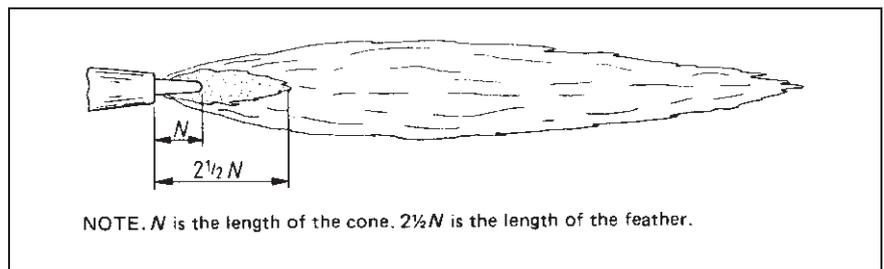
Figure 79 Oxidizing oxy-acetylene flame
