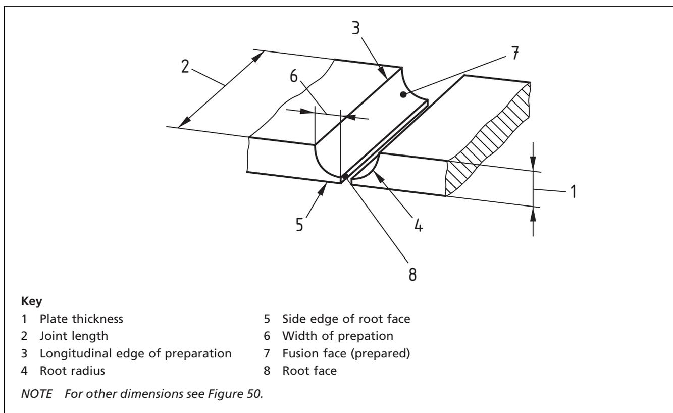
Figure 66 Typical example of fusion weld – Single V-butt weld
