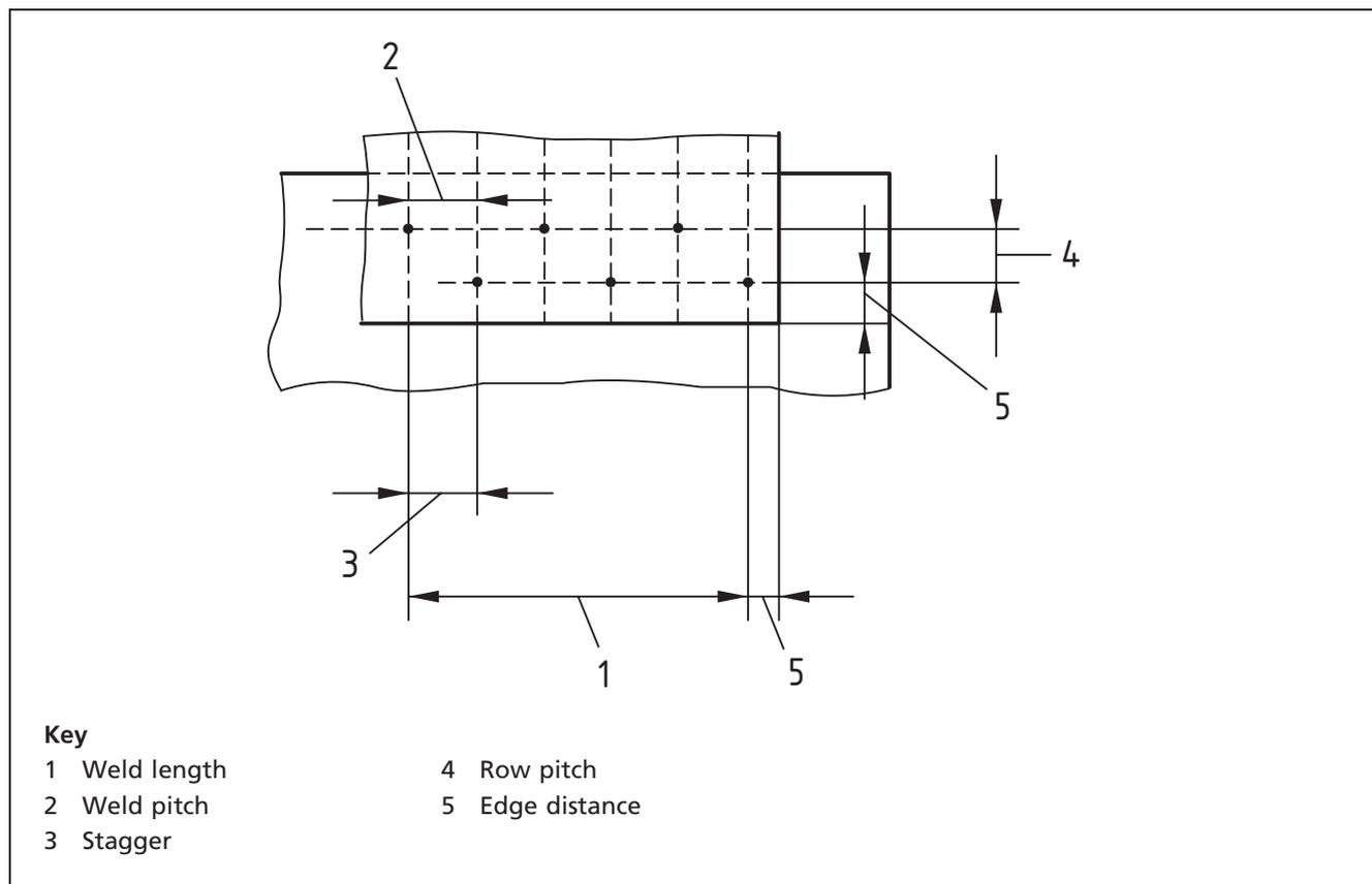
Figure 15 Typical example of weld made using pressure – Projection weld
