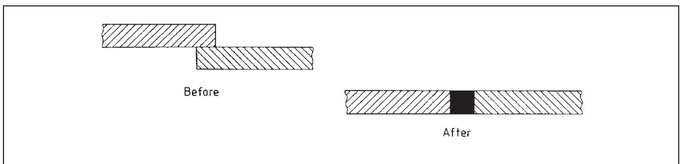
Figure 21 Nail head welding
