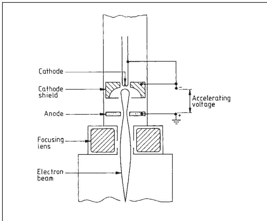
Figure 84 Diagrammatic representation of a triode gun
