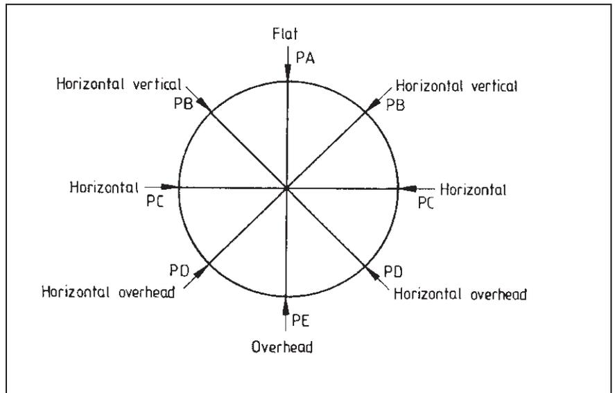
Figure 58 Comparison of UK (USA) and ISO welding positions
