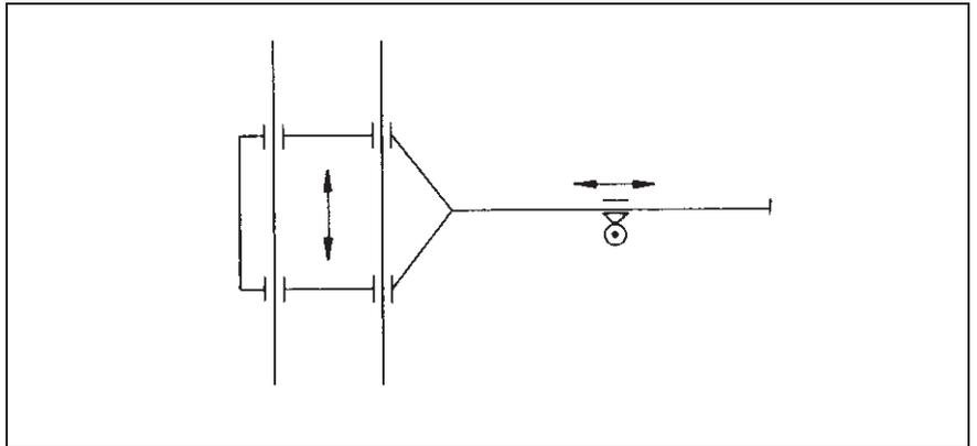
Figure 107 Double-cantilever cutting machine
