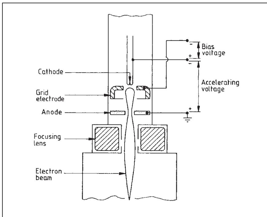
Figure 85 Diagrammatic representation of a back-bombarded gun
