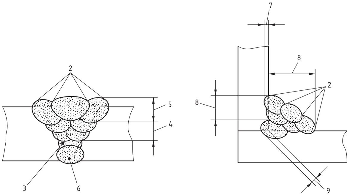
c) Single V-butt weld with sealing run
