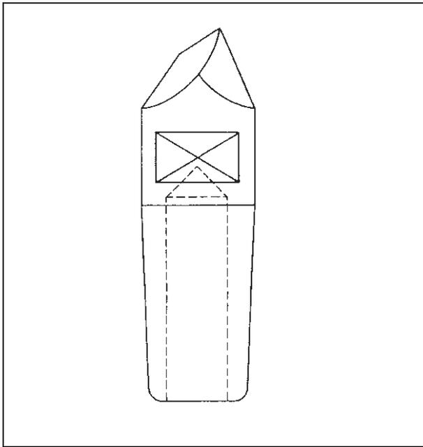
Figure 25 Cranked offset electrode
