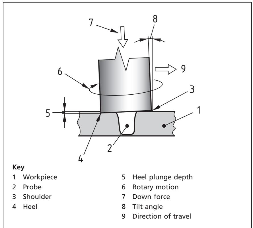
Figure 43 Adjustable probe tool
