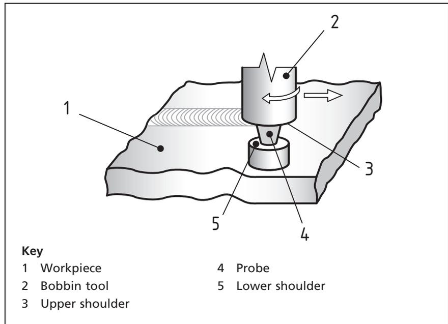
Figure 45 Self-reacting bobbin tool
