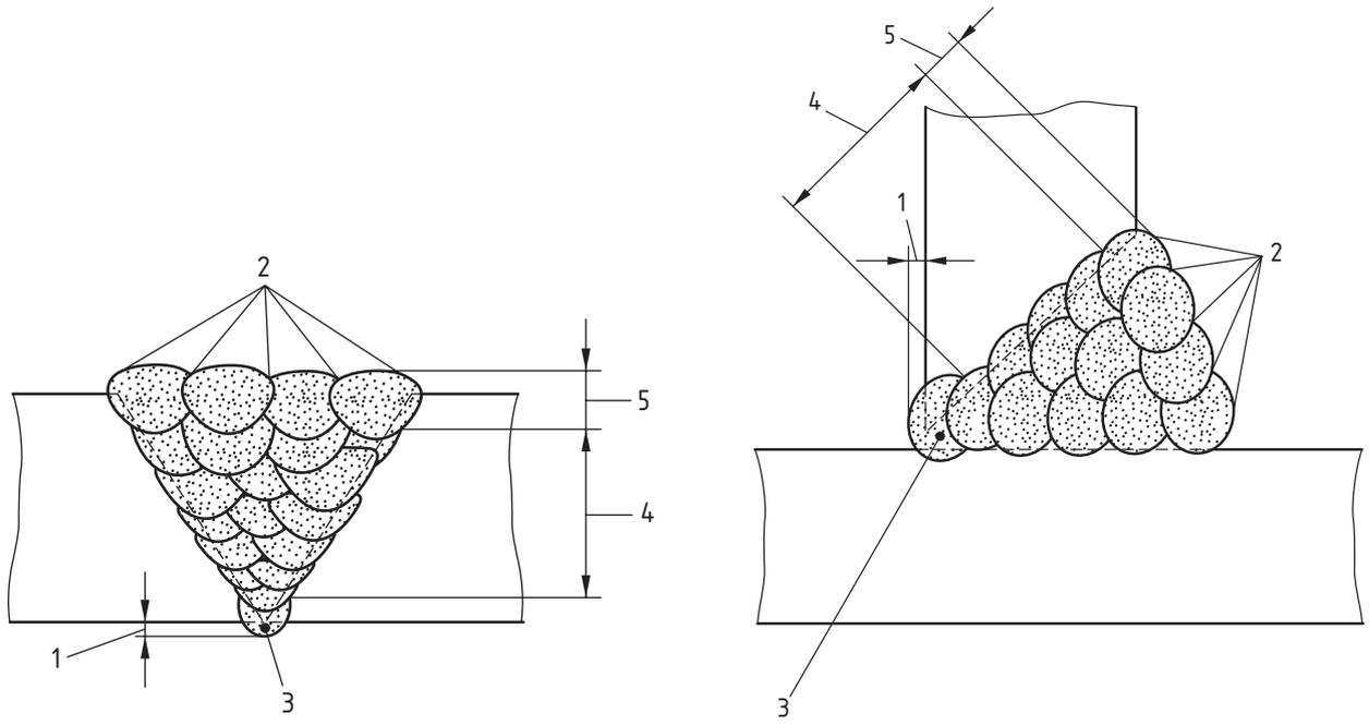
a) Single V-butt weld with root face
