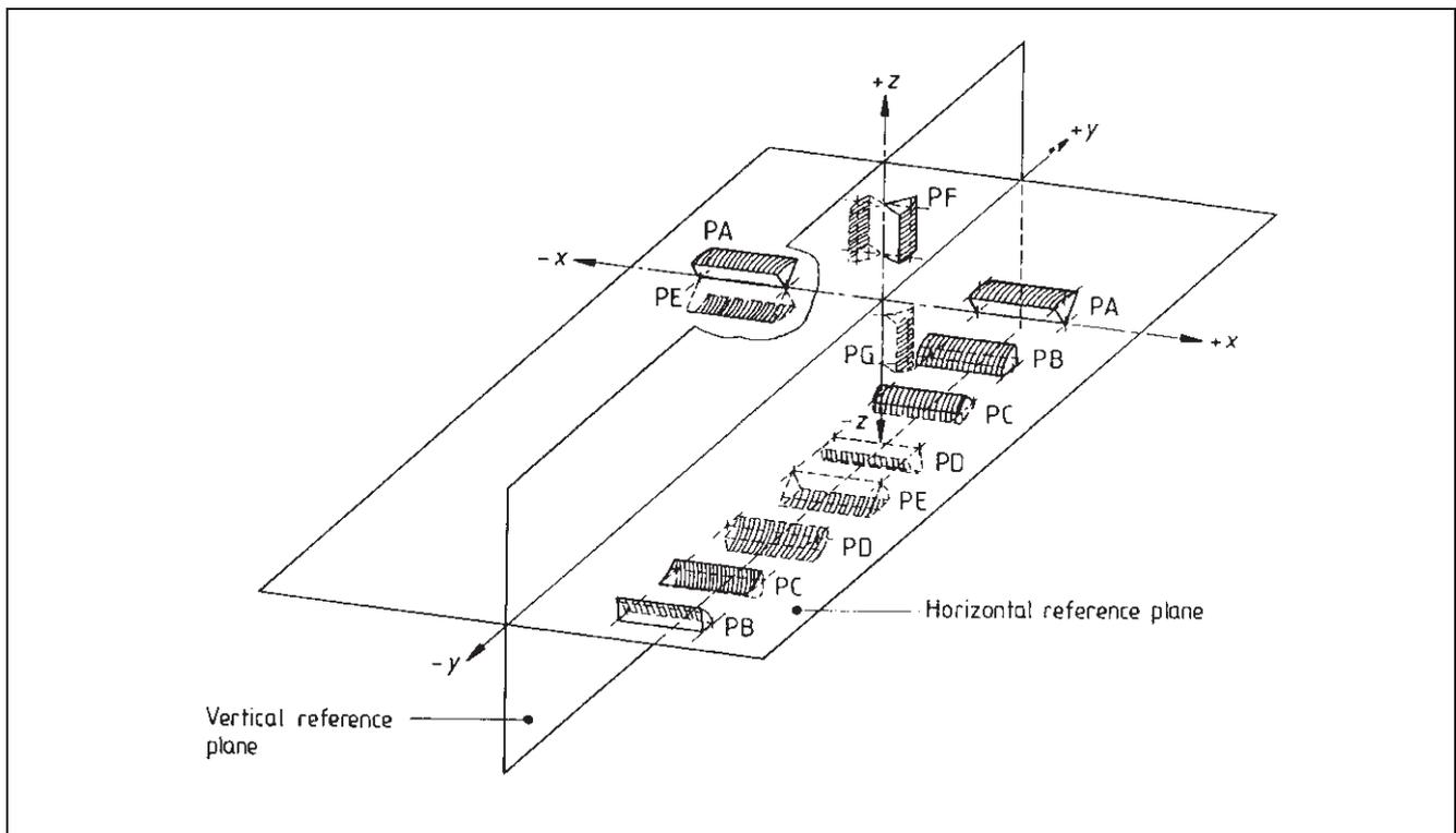
Figure 57 Simplified view of main welding positions
