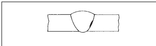
Figure 99 **Lack of root fusion**
